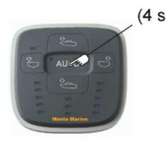
Run the boat at cruising speed. Manually control the trim tabs until you find the best attitude. Then, press and hold the auto button for 4 s until the AUTO indicator is lit up.
