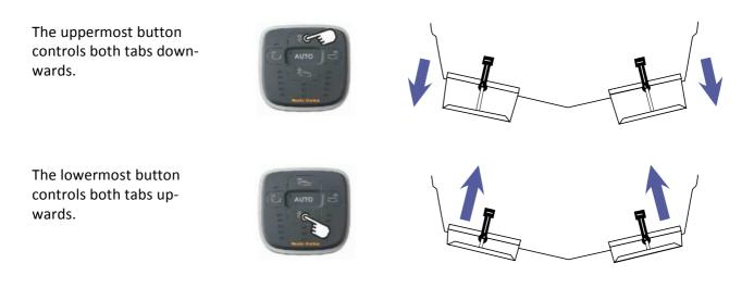
Should the trim tabs move in the wrong direction: For hydraulic trim tabs, exchange the 5 and 6 wires, for electromechanical trim tabs, reverse the wires of the actuator(s) that move in the wrong direction.
