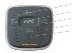
Light sensor (Optimum visibility day and night) Auto button with indicator (Auto / Manual mode) 4 x buttons for manual control of the trim tabs LED indicator bars for trim tab position LED indicator bar for gain setting
