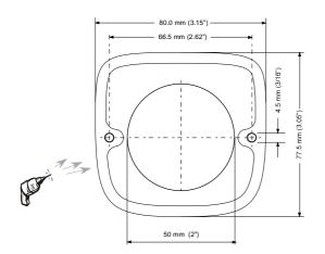
Choose a location close to the helm where the control panel is easy to access and drill holes for the screws and connectors using the enclosed drill pattern. In retrofit installations, remove the old panel and use the new panel to cover the hole.
