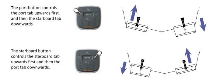
Should the trim tabs move in the wrong direction: For hydraulic trim tabs, exchange the 3 and 4 wires, for electromechanical trim tabs, exchange the 3 and 4 wires with the 5 and 6 wires.
